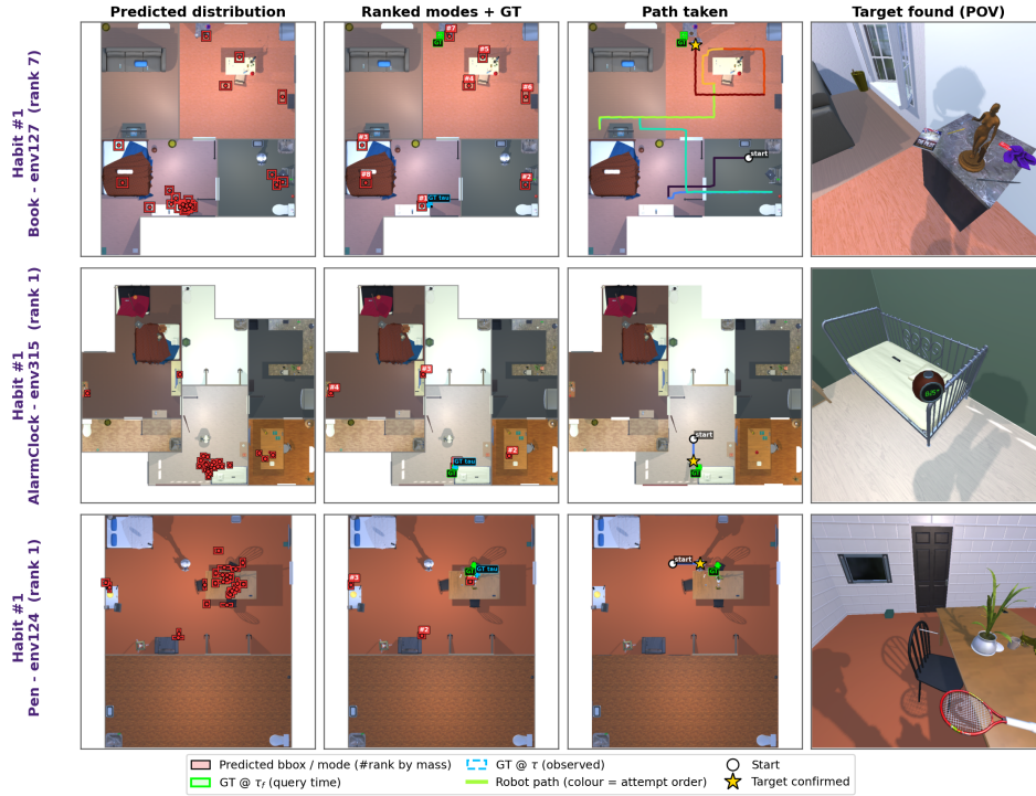
Figure 14: Representative successful ObjNav episodes with FlowMaps, set 7. Each row shows the predicted samples, ranked clusters, executed trajectory, and final target confirmation view.
